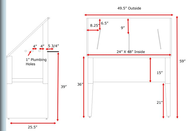
Available as Left, Right or center drain. 3.5" drain hole, located 7" on center from the left or right. (12" from front of tub and 12" from the back of the tub)
