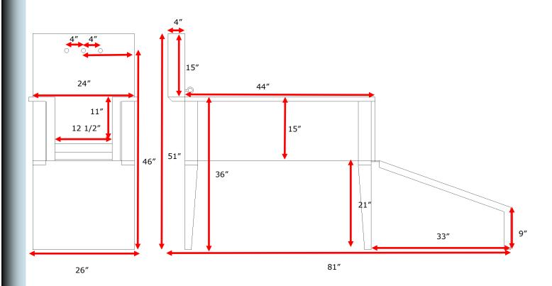
Available as Left, Right or center drain. 3.5'' drain hole, located 7'' on center from the back wall.
