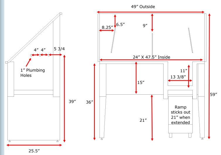
Faucet holes and drain are available on the left, right or center. Ramp is located on the opposite side of drain.
