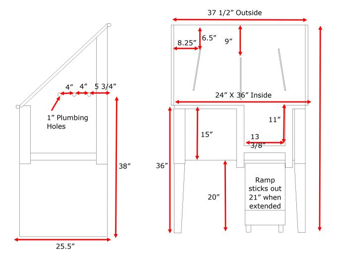
Faucet holes and drain are available on the left, right or center. Ramp is located on the opposite side of drain.
