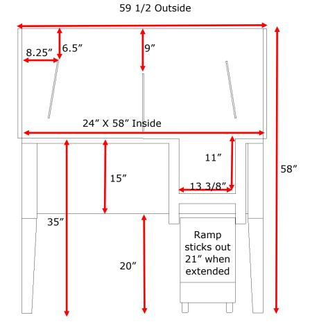
Faucet holes and drain are available on the left, right or center. Ramp is located on the opposite side of drain.
