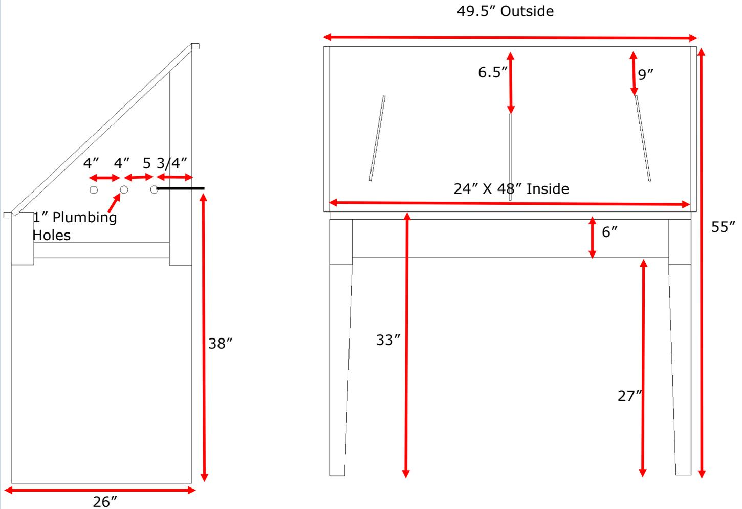
Available as Left, Right or center drain. 3.5" drain hole, located 7" on center from the left or right.
