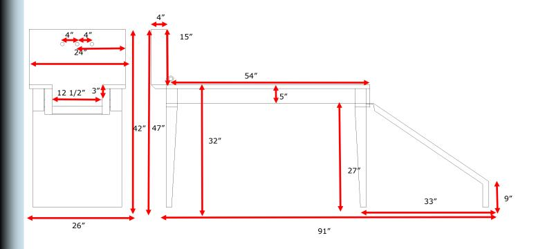
Available as Left, Right or center drain. 3.5" drain hole, located 7" on center from the back wall.
