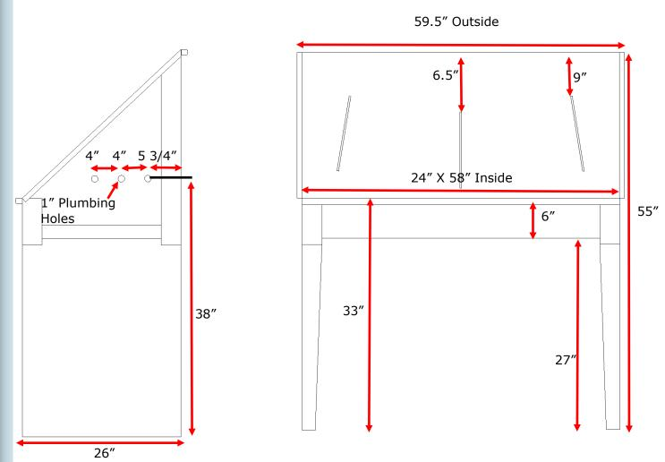
Available as Left, Right or center drain. 3.5" drain hole, located 7" on center from the left or right.
